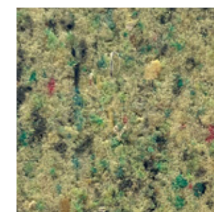
2,5 mm linoleum + 1,5 mm recycled foam
